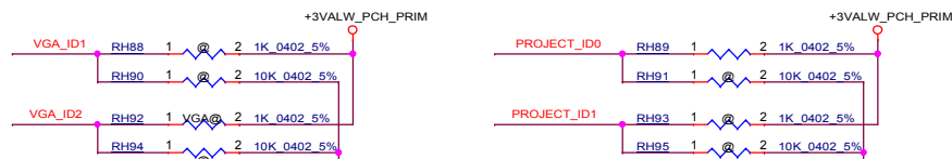
VGA_ID1 / VGA_ID2 / Project_ID0 / Project_ID1 SW set GPI interanl pull down 20K.
